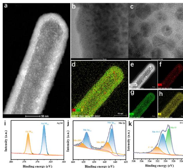
**Fig. 2** Fine-structure characterizations of Ag@MnO<sub>2</sub>: (a–c) HRTEM images; HAADF images: (d) the overlay image and elemental mapping images of (e) Ag, (f) Mn, and (g) O; high-resolution (h) Ag 2d XPS spectrum, (i) Mn 2p XPS spectrum, and (j) O 2p XPS spectrum, (k) O 1s XPS spectrum.
