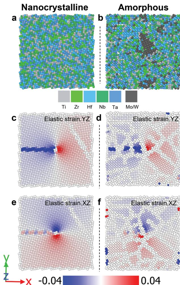
**Fig. 7** The schematics of (a) nanocrystalline and (b) amorphous materials after introducing a  $\frac{1}{2}$  [111] screw dislocation at the center and the corresponding elastic strain fields at (c and d) YZ and (e and f) XZ planes.
