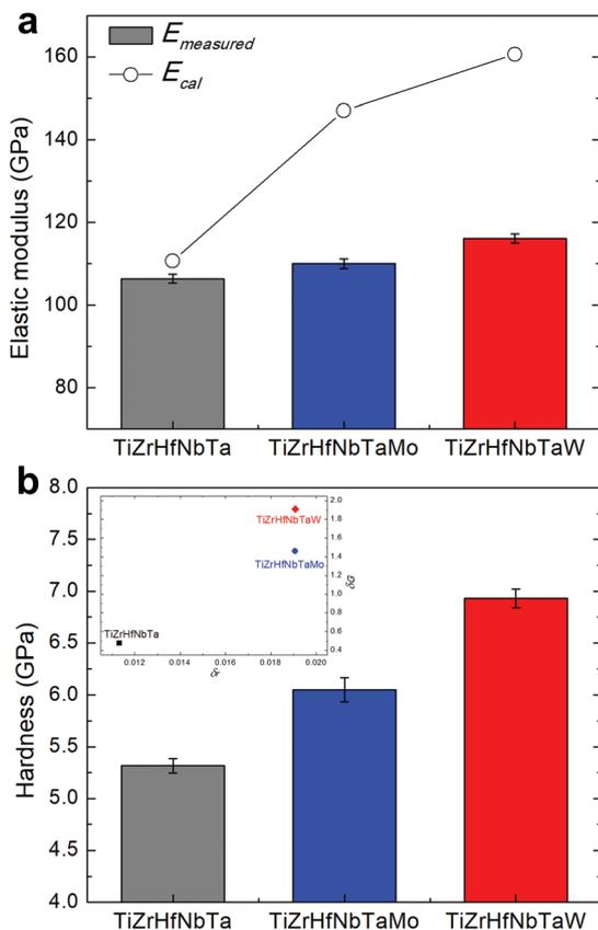
**Fig. 6** The nanoindentation measured (a) elastic moduli and (b) hardness of TiZrHfNbTa, TiZrHfNbTaMo, and TiZrHfNbTaW. The open circles in (a) indicate the calculated values based on the rule of mixtures. The inserted figure in (b) presents the calculated mismatches of shear modulus  $\delta_G$  and atomic size  $\delta_r$ .
