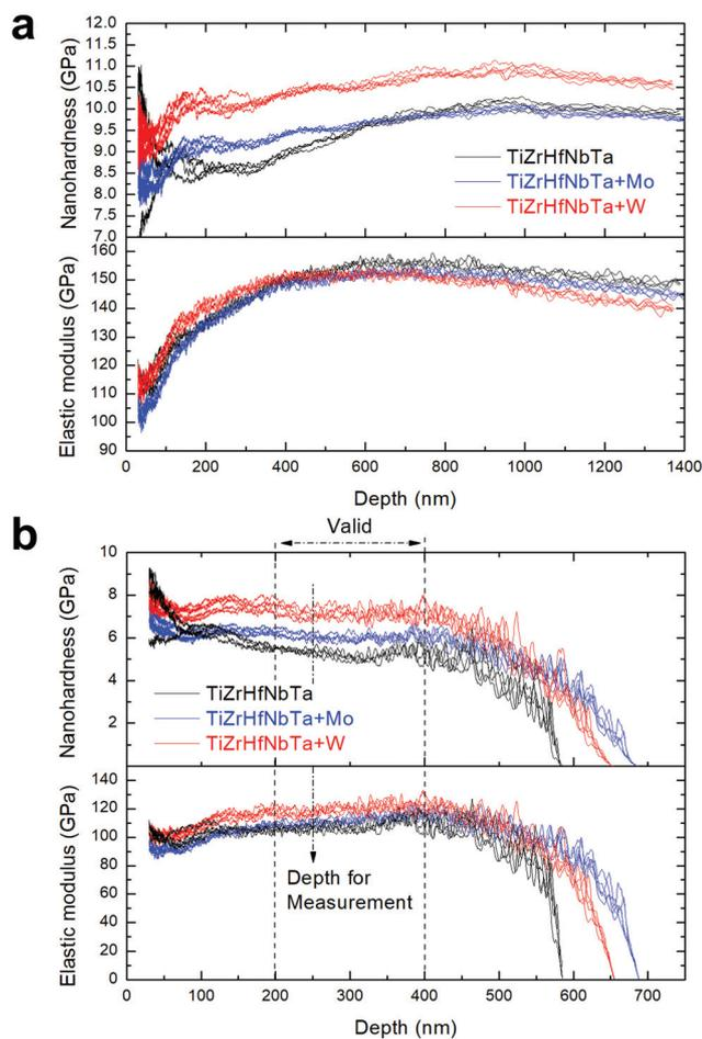
**Fig. 4** (a) Nanohardness and elastic modulus as functions of the depth in the as-deposited HEA thin films. (b) The corrected nanohardness and elastic modulus based on the modified King's model.<sup>27</sup> A depth of 250 nm is selected for further measurement.
