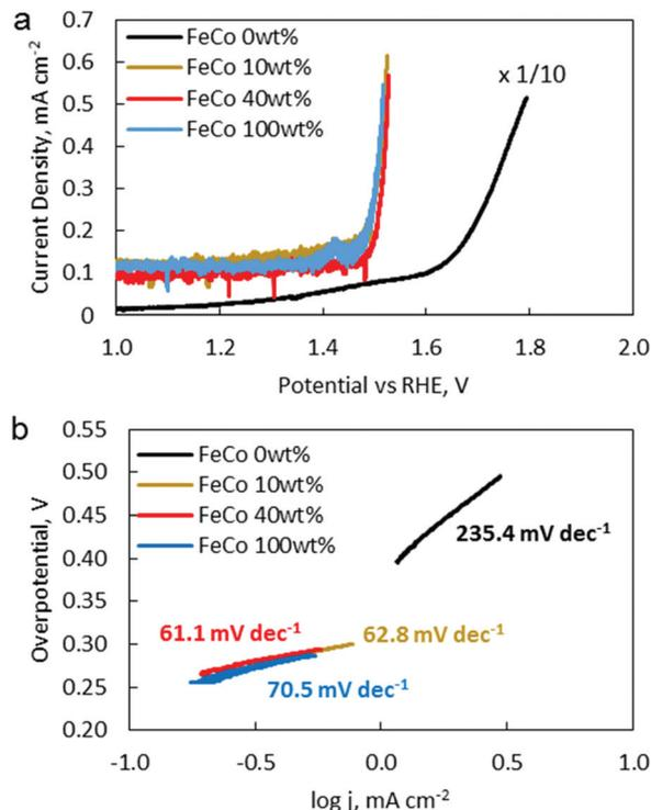
**Fig. 9** (a) LSVs of FeCo 0 wt% (black), FeCo 10 wt% (gold), FeCo 40 wt% (red), and FeCo 100 wt% (blue) from 1.0 V to the onset of the OER, in 1.0 M KOH, sat. Ar, at 1600 rpm, at a scan rate of  $1 \text{ mV s}^{-1}$ . (b) Tafel slopes derived from polarisation curves in (a). Overpotential is calculated from the thermodynamic potential of the OER (1.23 V vs. SHE).
