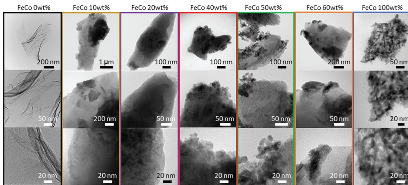
**Fig. 4** TEM micrographs in increasing magnification from the top to bottom of FeCo 0 wt% (black), FeCo 10 wt% (brown), FeCo 20 wt% (purple), FeCo 40 wt% (red), FeCo 50 wt% (green), FeCo 60 wt% (orange), and FeCo 100 wt% (blue) samples.
