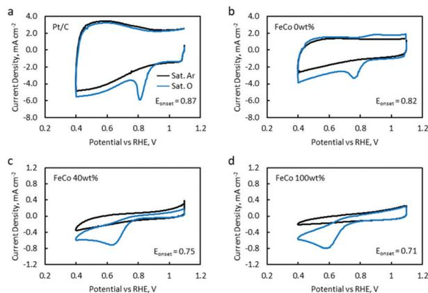
**Fig. 10** CVs of (a) a Pt/C reference, (b) FeCo 0 wt%, (c) FeCo 40 wt% and (d) FeCo 100 wt% in a saturated Ar electrolyte (black line) and a saturated  $\text{O}_2$  electrolyte (blue line). Scan rate was  $50 \text{ mV s}^{-1}$ , in 1.0 M KOH with a stationary RDE.
