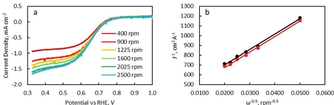
**Fig. 11** (a) LSV of FeCo 40 wt% at a RDE rotation speed of 400 rpm (dark red), 900 rpm (red), 1225 rpm (yellow), 1600 rpm (light green), 2025 rpm (green) and 2500 rpm (blue). (b) A K-L plot of polarisation curves from LSV at 0.45 V (red) and 0.50 V (black).
