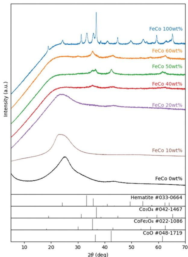
**Fig. 3** XRD patterns of FeCo 0 wt% (black), FeCo 10 wt% (brown), FeCo 20 wt% (purple), FeCo 40 wt% (red), FeCo 50 wt% (green), FeCo 60 wt% (orange), and FeCo 100 wt% (blue) samples after sintering. Reference patterns of CoO (JCPDF #048-1719),  $\text{CoFe}_2\text{O}_4$  (JCPDF #022-1086),  $\text{Co}_3\text{O}_4$  (JCPDF #042-1467), and hematite  $\text{Fe}_2\text{O}_3$  (JCPDF #033-0664) are provided in stick forms.
