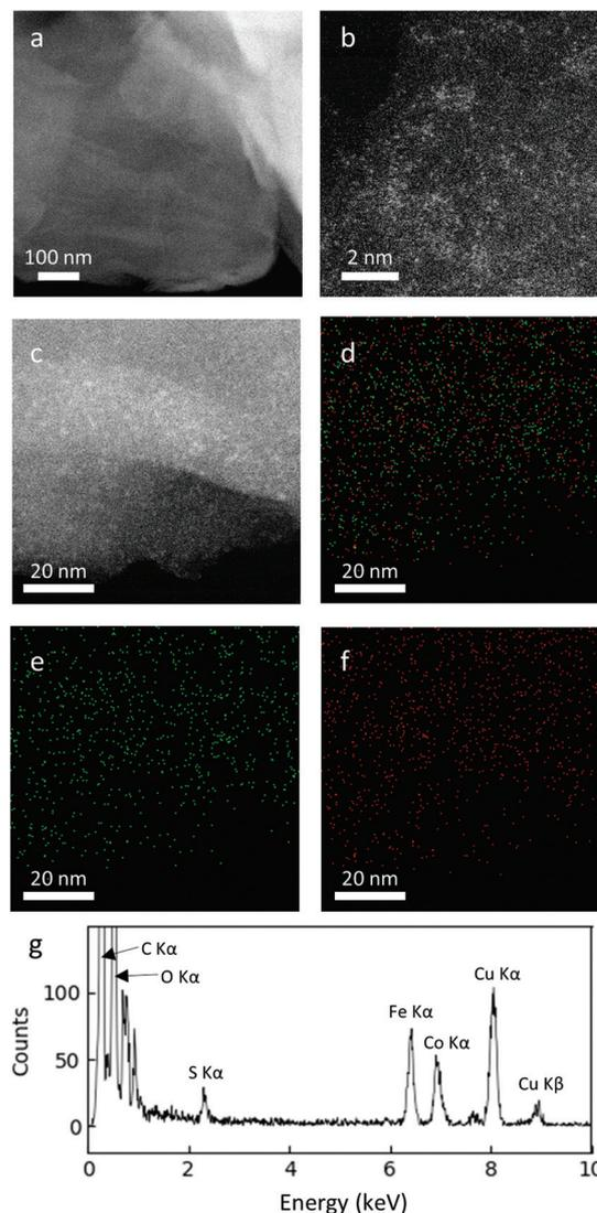
**Fig. 6** STEM micrographs of FeCo 10 wt%. (a–c) HAADF images at various magnifications. (c) Area used for EDS element mapping. (d) Overlay of Fe K (red) and Co K (green). (e) Element map for Co K (green). (f) Element map for Fe K (red). (g) EDS spectrum of the mapped area.
