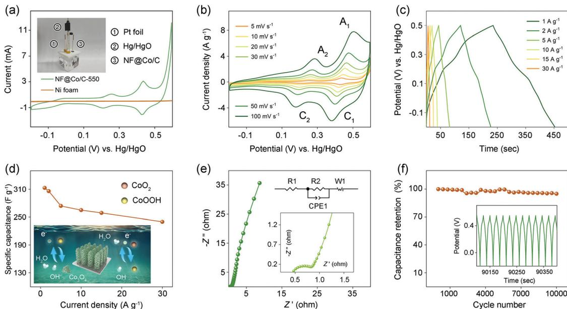
**Fig. 8** (a) CV curves of Ni foam and NF@Co/C-550 sample at a scan rate of  $5 \text{ mV s}^{-1}$ . Inset is a three-electrode system. (b) CV curves of NF@Co/C-550 sample at different scan rates. (c) GCD curves at different current densities. (d) Specific capacitance. Inset is the schematic illustration for electrode reaction. (e) Nyquist plots and the corresponding equivalent circuit. (f) Cycling performance at a charge–discharge current density of  $10 \text{ A g}^{-1}$ .
