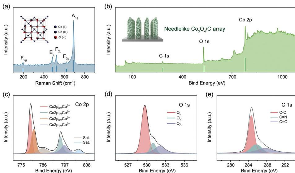
**Fig. 4** (a) Raman spectrum of NF@Co/C, and inset is the crystal structure of  $\text{Co}_3\text{O}_4$ . (b) Broad scan XPS spectrum of NF@Co/C, and inset is the corresponding model. (c) Co 2p spectrum. (d) O 1s spectrum. (e) C 1s spectrum.
