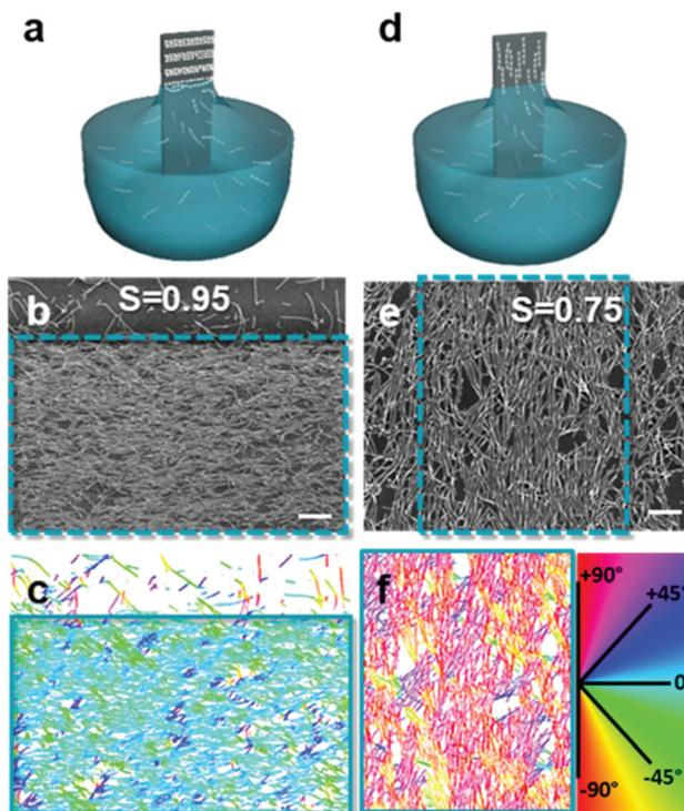
**Fig. 7** Assembly in the (a) convective and (d) Landau–Levich regimes, where the (b and e) degree of disorder between assembled helices varies. (c and f) The order parameter,  $S$ , was obtained by treating the images to determine the orientation of the helices relative to the withdrawal direction. Scale bars represent 1  $\mu\text{m}$ . Reproduced with permission from ref. 102. Copyright 2020 American Chemical Society.
