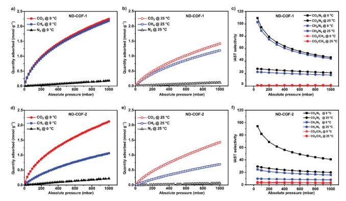
Fig. 3 Gas adsorption and selectivity data for the ND-COFs. ND-COF-1:  $CO_2$ ,  $CH_4$ , and  $N_2$  adsorption isotherms at (a) 0 °C and (b) 25 °C; (c)  $CO_2$ /  $N_2$ ,  $CH_4$ / $N_2$ , and  $CO_2$ / $CH_4$  ideal adsorbed solution theory (IAST) selectivity at 0 °C and 25 °C. ND-COF-2:  $CO_2$ ,  $CH_4$ , and  $CO_2$ / $CH_4$  and  $CO_2$ / $CH_4$  ideal adsorption isotherm at (d) 0 °C and (e) 25 °C; (f)  $CO_2$ / $CO_2$ /CO
