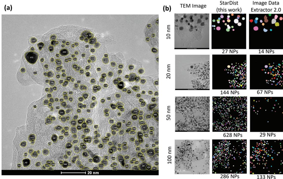
**Fig. 5** (a) Localization and counting the particles made available by the instance segmentation approach. (b) Comparison between the predicted segmentation maps of test images at different scales using the StarDist model employed in this work and the ImageDataExtractor 2.0.<sup>64</sup>
