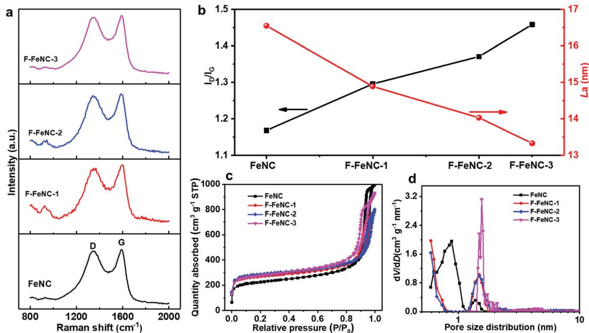
Fig. 2 (a) Raman spectra, (b)  $L_a$  sizes and the ratio of the G and D bands ( $I_D/I_G$ ) in the Raman spectra, (c)  $N_2$  adsorption/desorption isotherms and (d) pore size distributions processed from the non-local density functional theory (NLDFT) analysis FeNC, F-FeNC-1, F-FeNC-2, and F-FeNC-3.
