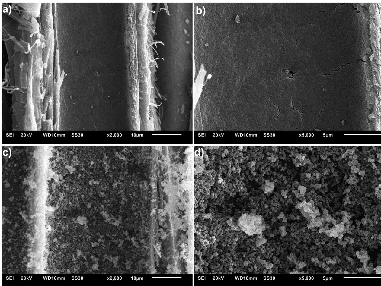
**Fig. 5** SEM images of cross sections of the composite materials with the highest MOF-loading. a) and b) MIL-53(Al)@Pine-MA. c) and d) ZIF-8@Pine-APTES. In both cases, the direction of the lumina channels is from top to bottom.
