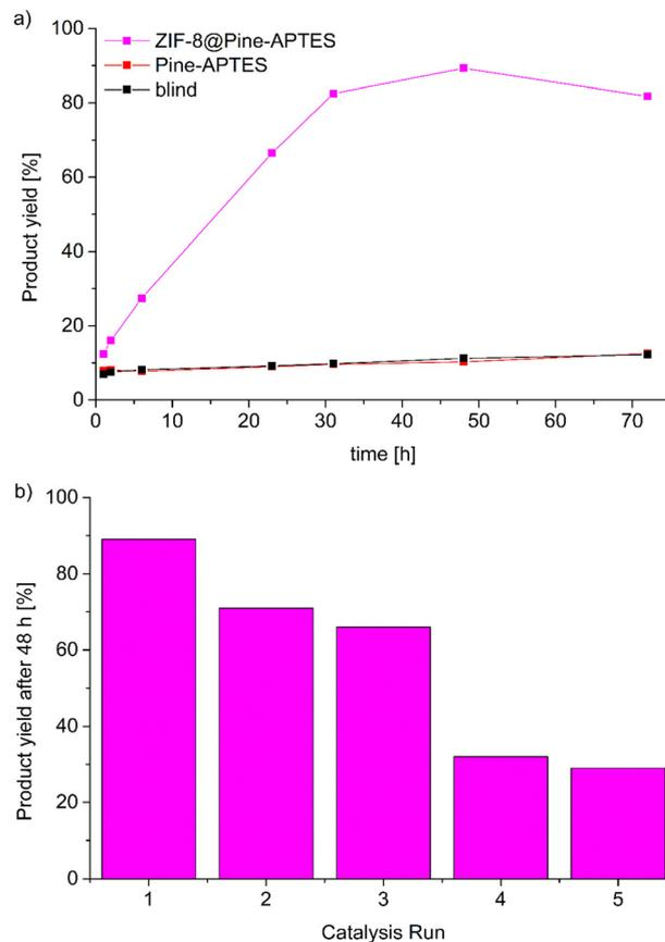
**Fig. 9** a) Product yield from the Knoevenagel condensation between benzaldehyde and malononitrile catalyzed by ZIF-8@Pine-APTES or Pine-APTES including the blind test without catalyst. b) Product yield for the catalysis with ZIF-8@Pine-APTES after 48 h over 5 reaction cycles.
