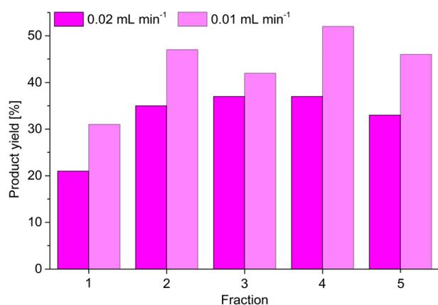
**Fig. 10** Results for continuous catalysis of the Knoevenagel condensation between benzaldehyde and malononitrile using ZIF-8@Pine-APTES as catalyst. One fraction is equal to 1 mL of precursor solution pushed out of the syringe.
