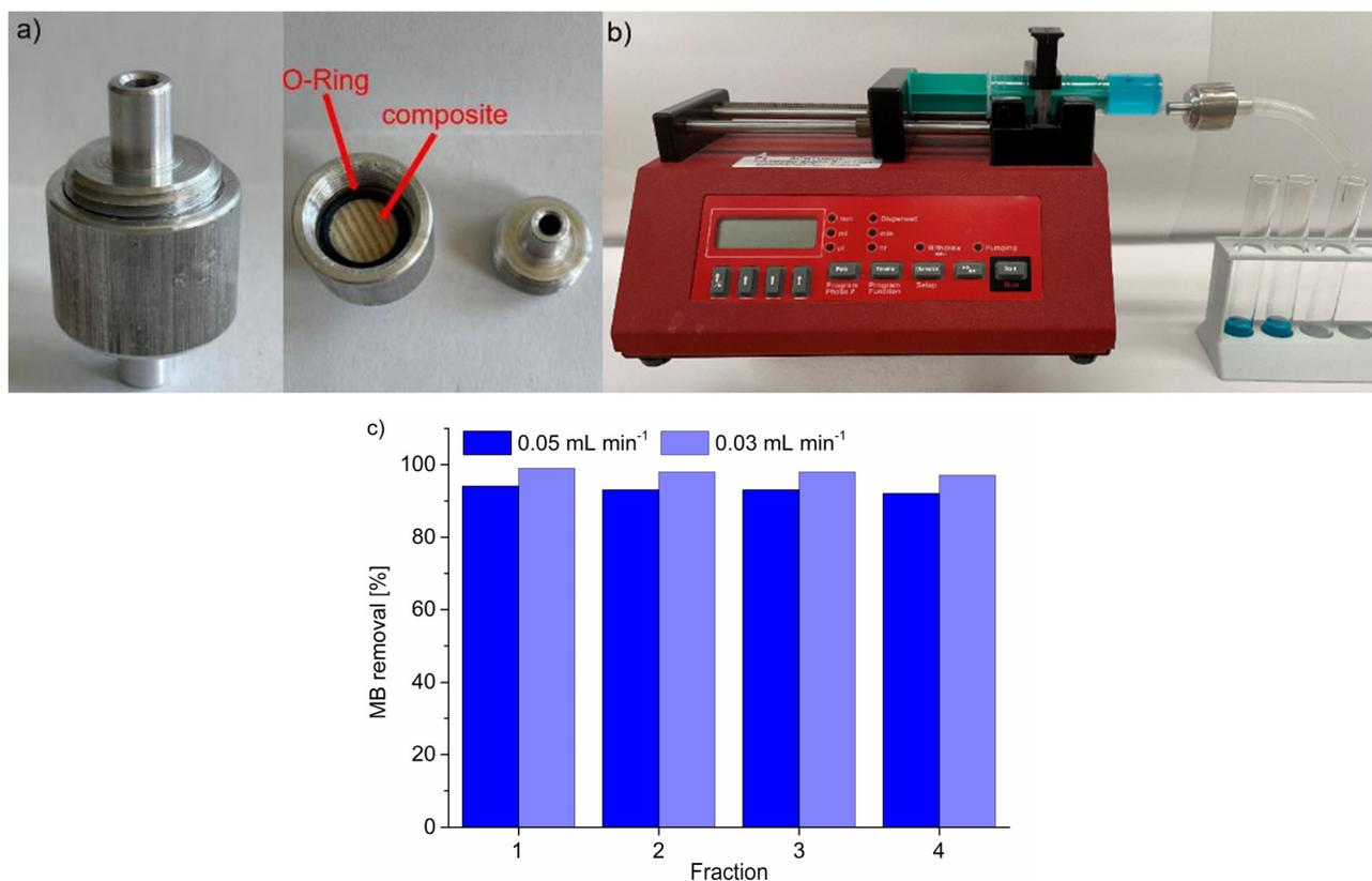
**Fig. 8** a) Custom-made filtration capsule used to mount the MOF@wood composite for continuous filtration/catalysis. b) Setup for the continuous filtration/catalysis using a syringe pump and the custom-made filtration capsule. c) Results of the continuous filtration of MB from aqueous solution using MIL-53(Al)@Pine-MA. One fraction is equal to 5 mL of MB solution pushed out of the syringe.
