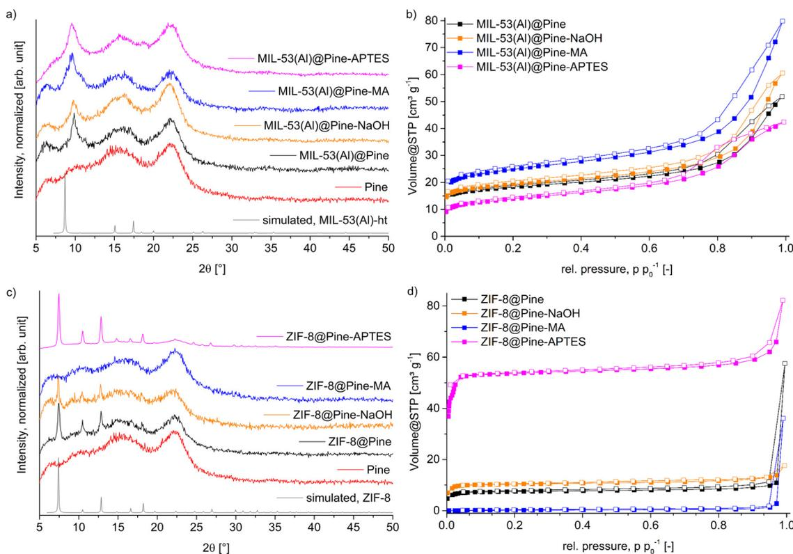
**Fig. 4** a) and c) PXRD patterns of MIL-53(Al) and ZIF-8@wood composite materials. Simulated patterns were obtained from the crystal structures of MIL-53(Al) (CSD-Refcode: SABVUN01)<sup>57</sup> and ZIF-8 (CSD-Refcode: FAWCEN).<sup>61</sup> b) and d) Nitrogen-sorption isotherms (at  $77 \text{ K}$ ) of MIL-53(Al) and ZIF-8@wood composite materials. For nitrogen-sorption isotherms, the filled symbols represent the adsorption branch, while the empty symbols represent the desorption branch.
