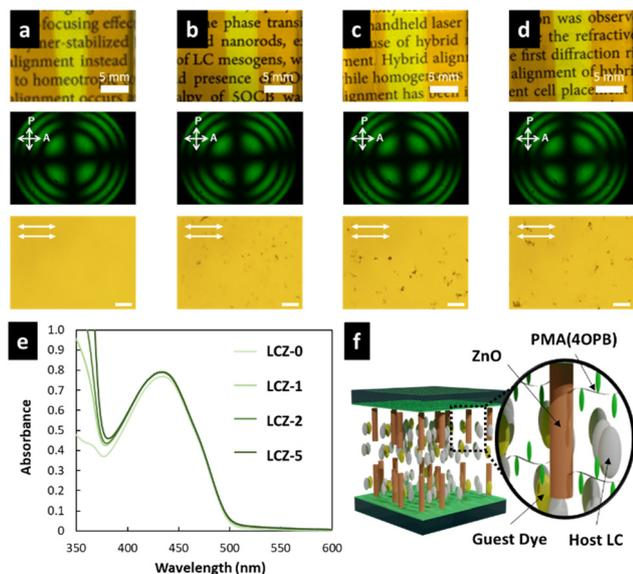
**Fig. 3** Orientation of TR5-doped host LC containing polymer-grafted nanorods. Photograph (top), conoscopic (middle), and orthoscopic (bottom) polarized optical micrographs observed with a 20 $\times$  objective lens of LC cells containing LCZ samples at the concentrations of 0 (a), 1 (b), 2 (c), and 5 (d) wt%. The scale bar is 50  $\mu\text{m}$ . (e) Polarized UV-vis absorption spectra for LCZ-X. (f) Schematic representation of TR5-doped LCs containing polymer-grafted nanorods.
