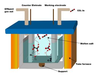
Fig. 1 Schematic of the MSCC-ET reactor.
