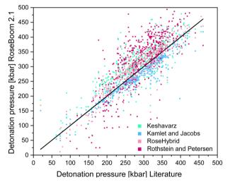
Scattering plot of the detonation pressures predicted with the methods implemented in RoseBoom2.1(), plotted against the literature values.
