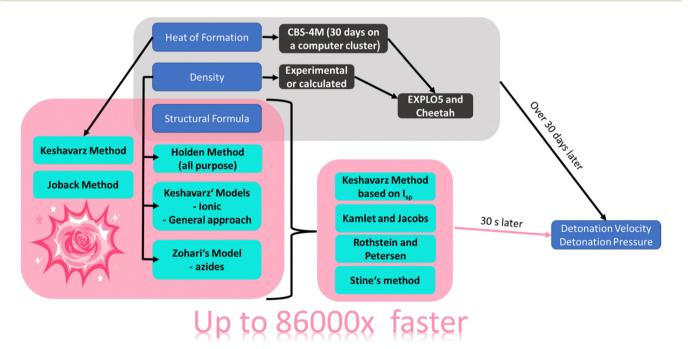
Fig. 3 Schematic overview of the methods which are currently commonly used (grey) to predict the detonation parameters, as well as the approaches take in this work (pink), along with durations required for the two different methods.
