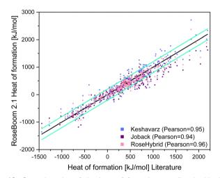
Fig. 10 Scattering plot of the heat of formations predicted with the methods implemented in RoseBoom2.1(C), plotted against the literature values, with turquoise error bars marking a range of  $\pm 200 \text{ kJ mol}^{-1}$
