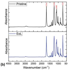
Fig. 4 FTIR spectra for (a) the inner surface of and (b) the outer surface of pristine and EoL pouches. The inner surfaces give spectra that are consistent with a polypropylene surface, while the outer surfaces' spectra are consistent with a PET material.
