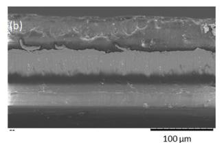
Fig. 2 (a) Schematic diagram of a layered pouch film (b) SEM image of a cross section through a pouch film, showing the layered structure.
