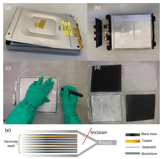
Fig. 1 (a) Photograph of a battery module, containing 4 cells. (b) Photograph of a cell having been removed from a module. (c) Photograph of an incision being made into the edge of a cell. (d) Photograph showing the separated parts of the cell (e) diagram to show the components of the pouch cell.
