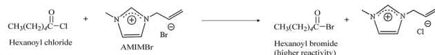
Fig. 13 Halogen exchange reaction between hexanoyl chloride and AMIMBr to produce hexanoyl bromide (reprinted with permission from ref. 119. Copyright 2021 Elsevier; DOI: 10.1016/j.ijbiomac.2021.09.044).
