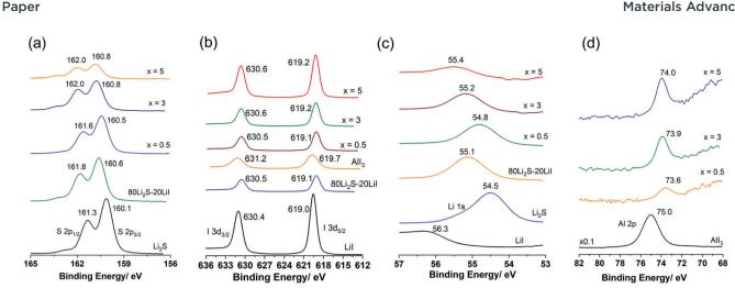
X-Ray photoelectron spectroscopy spectra (envelope) of the prepared samples and standard materials. (a) S 2p; (b) I 3d; (c) Li 1s; and (d) Al 2p.
