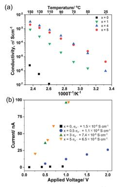
Fig. 4 Temperature dependence of ionic conductivity (a) and I-V correlation (polarized electronic current) (b) of  $(100 - x)Li_2S - xAll_3$ .
