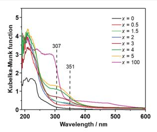
Fig. 2 UV-Vis spectra of  $\text{Li}_2\text{S}$  (x = 0), All<sub>3</sub> (x = 100), and (100 - x) $\text{Li}_2\text{S}$ -xAll<sub>3</sub>
