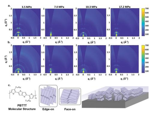
Fig. 3 GIWAXS patterns of PBTTT- $C_{14}$  films grown in (a) n-pentane and (b) n-pentane: toluene at different pressures. (c) The molecular structure of PBTTT-C<sub>14</sub> and the drawing illustrating the different molecular orientation of PBTTT-C<sub>14</sub> (edge-on and face-on) in thin layers with respect to the substrate surface
