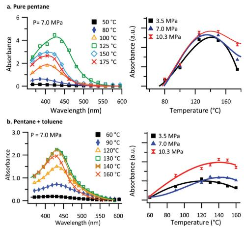
Fig. 1 In situ UV-vis transmission results of PBTTT- $C_{14}$  in (a) pure n-pentane and (b) n-pentane: toluene (0.5% mol) solution. UV-vis spectral measurements for the chamber and its contents (solution) for several temperatures and a single pressure (left) and the integrated UV-vis absorbance as a function of temperature for several pressures (right). Solid lines indicate the fit to the data using eqn (1).
