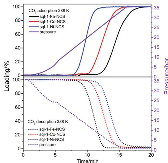
Fig. 4 Kinetics of CO<sub>2</sub> adsorption (top) and desorption (bottom) for **sql-1-M-NCS** (M = Fe, Co and Ni) at 288 K.
