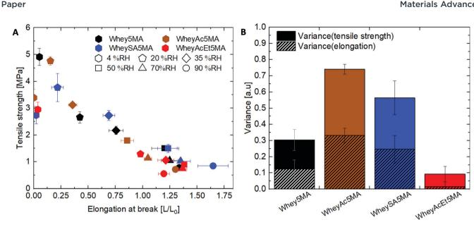
Fig. 6 (A) Elongation at break and ultimate tensile strength of copolymers equilibrated at relative humidity levels ranging from 4–90% RH. Copolymers are color coded based on the type of protein modification, and the equilibration conditions are noted with different marker shapes. Copolymers with small mechanical property variations with humidity are clustered closer together. (B) Data clustering from 20-90% RH determined as the variance.
