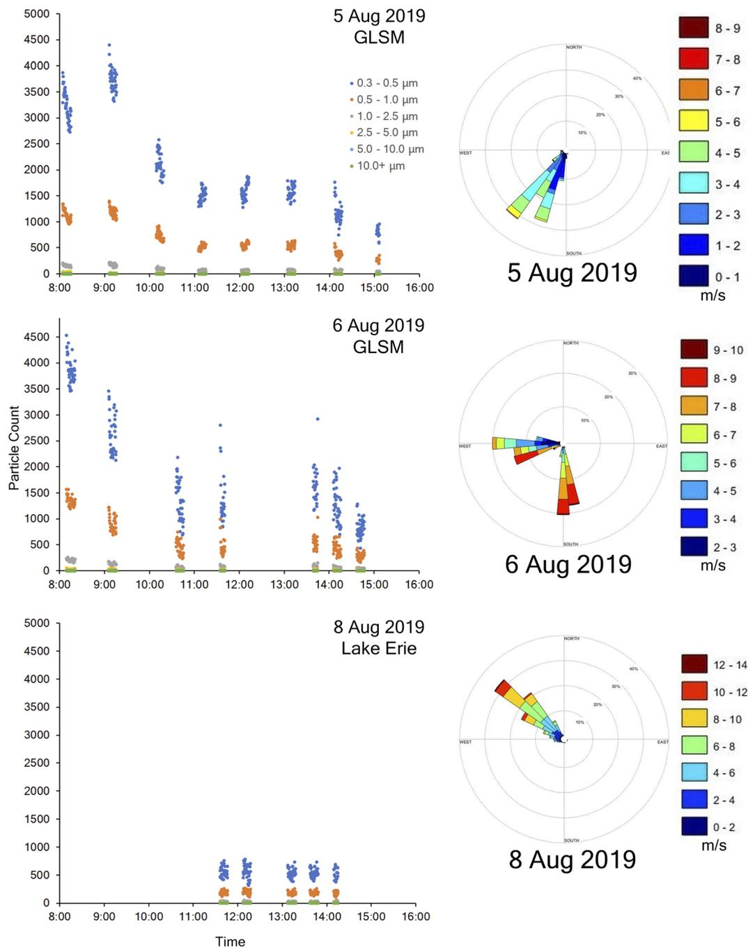
Fig. 5 Airborne particle counts over the course of the day. Data were recorded from a PMS7003 OPC onboard the AirDROPS. The first two graphs show flights that occurred August 5<sup>th</sup> to 6<sup>th</sup>, 2019 at GLSM while hovering 10 m over the water. The third graph depicts the flights on August 8<sup>th</sup>, 2019 while hovering 10 meters over the water at LE. To the right of each graph is the corresponding wind rose which shows wind direction and speed ( $\text{m s}^{-1}$ ) each day.
