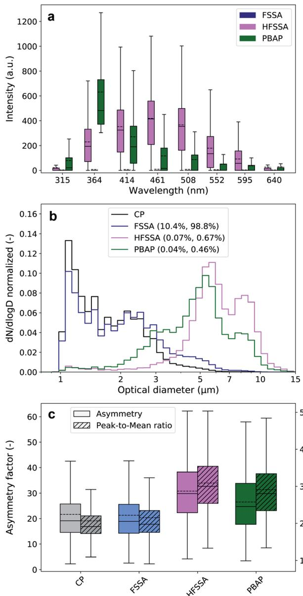
**Fig. 3** Result of decision tree classification of all fluorescent particles. (a) Fluorescence spectra of the different fluorescent particle groups. (b) Integral-normalized size distributions with their overall contribution to the measured coarse particles and fluorescent particles given in the legend, respectively. The black line denotes the normalized size distribution of all coarse particles (CP). (c) The asymmetry and peak-to-mean ratio of fluorescent groups and all CP.
