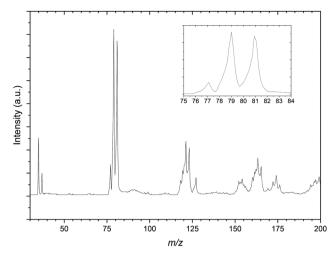
Fig. 2 Mass spectrum resulting from the CH<sub>2</sub>Br<sub>2</sub>:C<sub>3</sub>H<sub>6</sub>:Ar gas mixture. The spectrum shows mass peaks resulting from the bare Cl<sup>-</sup> anions and propene complexes with Cl<sup>-</sup> and Br<sup>-</sup>. Inset: The bare Br<sup>-</sup> is isobaric with the  ${}^{37}Cl^-\cdots C_3H_6$  complex.
