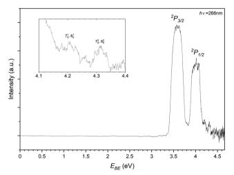
Fig. 6 Photoelectron spectrum of the 123 m/z peak from Fig. 2 assigned to photodetachment to the perturbed  ${}^{2}P_{3/2}$  and  ${}^{2}P_{1/2}$  states of the  $Br^- \cdots C_3 H_6$  complex.
