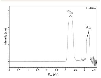
Fig. 8 Photoelectron spectrum of the 169 m/z peak from Fig. 3 assigned to photodetachment to the perturbed  ${}^2P_{3/2}$  and  ${}^2P_{1/2}$  states of the
