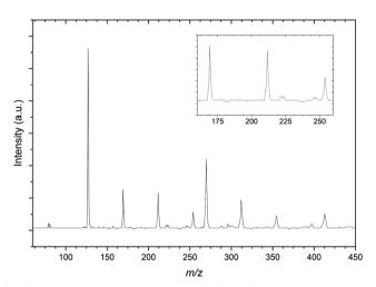
Fig. 3 Mass spectrum resulting from the CH<sub>3</sub>I:C<sub>3</sub>H<sub>6</sub>:Ar gas mixture. The spectrum shows mass peaks resulting from the bare Br- anions and propene complexes with I<sup>-</sup>. Inset: Highlighted the peaks at 169, 211 and 254 m/z assigned to the  $I^- \cdots (C_3 H_6)_n$  (n = 1-3) complexes.
