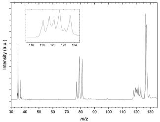
Fig. 4 Mass spectrum resulting from the CCl<sub>4</sub>:C<sub>3</sub>H<sub>6</sub>:Ar gas mixture. The spectrum shows mass peaks resulting from the bare halides and propene complexes with both Cl<sup>-</sup> and Br<sup>-</sup>. Inset: Highlighted the peaks at 118-124 m/z assigned to the Br $^-\cdots$ C<sub>3</sub>H<sub>6</sub> and Cl $^-\cdots$ (C<sub>3</sub>H<sub>6</sub>)<sub>2</sub> complexes.
