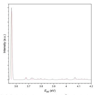
Fig. 7 Simulated photoelectron spectrum for the  ${}^2P_{3/2}$  photodetachment of the  $Br^- \cdots C_3H_6$  complex. Stick spectra (red) represent the individual FCFs calculated. The black trace is a Gaussian convolution with width,  $\omega = 0.005$
