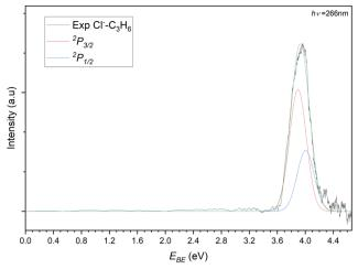
Fig. 5 Photoelectron spectrum of the 77 m/z peak from Fig. 4. The spectrum is deconvoluted into two gaussians representing the perturbed  $^2P_{3/2}$  (red) and  $^2P_{3/2}$  (blue) states of the Cl $^-\cdots$ C<sub>3</sub>H<sub>6</sub> complex
