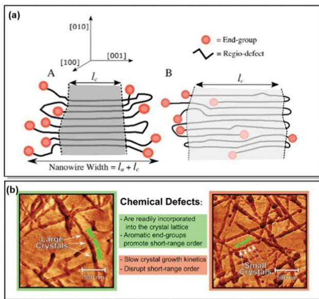
Fig. 3 (a) Proposed **P3HT** nanowire structures with (A) complete or (B) partial defect expulsion, where the darker grey area corresponds to the higher crystallinity region. (b) Young's modulus AFM scans of **P3HT** nanowires with lower (left panel) and higher (right panel) defect concentration. Reproduced with permission from American Chemical Society.<sup>70</sup>
