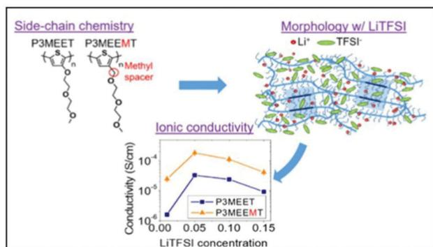
Fig. 6 Top-left panel: chemical structures of **P3MEET** and **P3MEEMT**. Top-right panel: Schematic representation of LiTFSI distribution within **P3MEET/P3MEEMT** semicrystalline structure at high concentration of LiTFSI. Bottom panel: **P3MEET** and **P3MEEMT** ionic conductivity at 90 °C. Reproduced with permission from American Chemical Society.<sup>81</sup>
