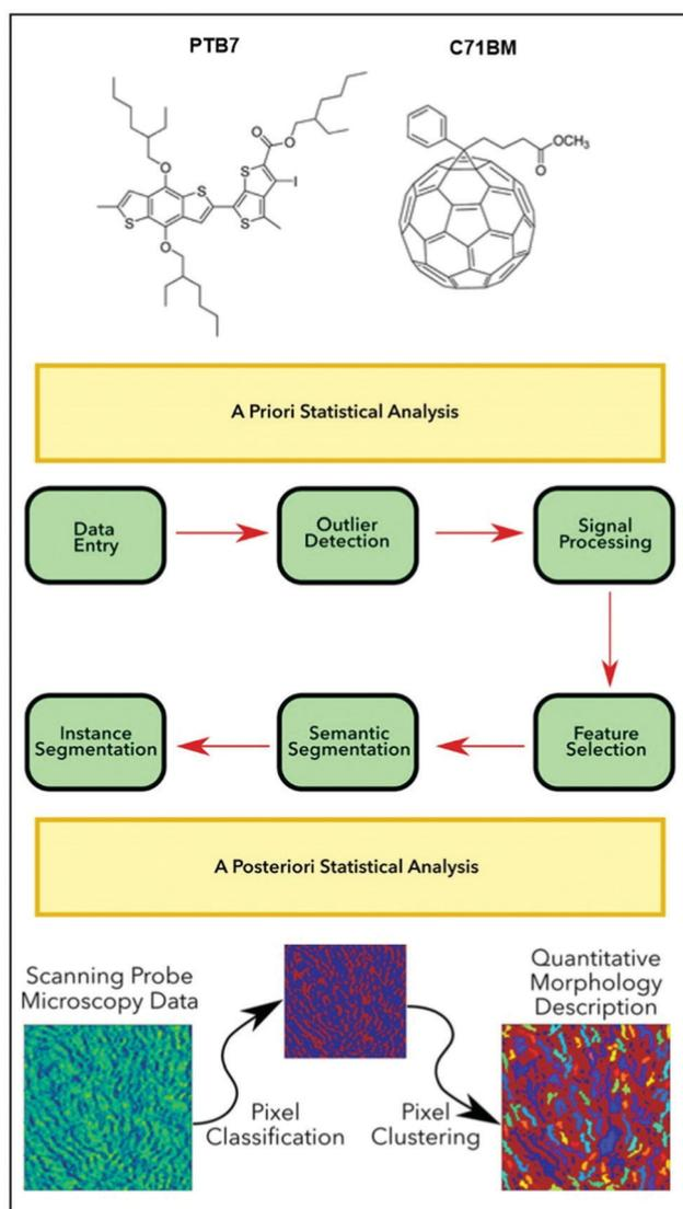
Fig. 12 Top panel: Chemical structures of (**PTB7**):**PC71BM**. Middle panel: A generalized m2py workflow. Bottom panel: Schematic of the recognition and visualization of the experimental SPM data by the m2py toolkit. Reproduced with permission from American Chemical Society.<sup>97</sup>
