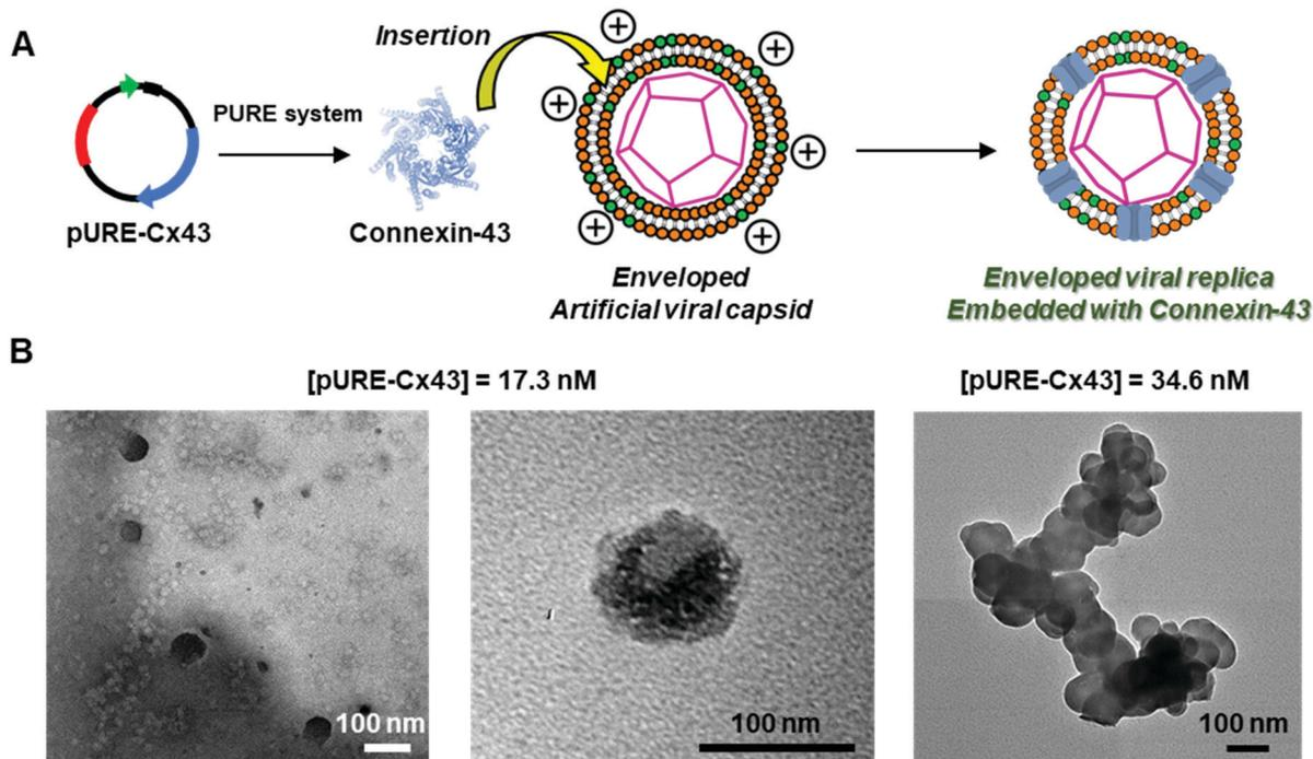
Fig. 1 (A) Schematic illustration and (B) TEM images of enveloped viral capsid embedded with Cx43 ( $[\beta\text{-annulus-EE}] = 16 \mu\text{M}$ ,  $[\text{DOTAP}] = 48 \mu\text{M}$ ,  $[\text{DOPC}] = 480 \mu\text{M}$ ). Cx43 was expressed from 17.3 to 34.6 nM pPURE-Cx43 using the PURE system. The samples were stained with EM stainer.
