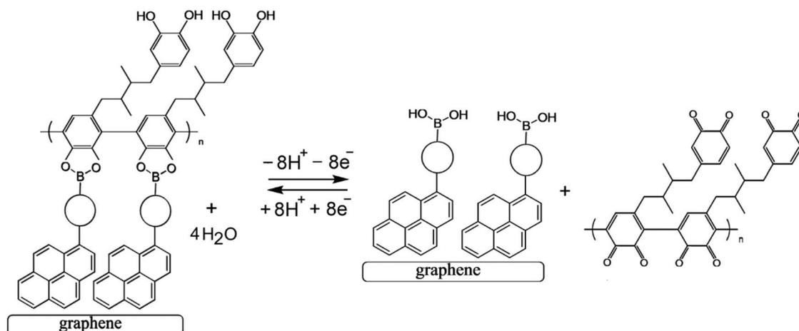
**Fig. 6** Illustration of Process 2 based on oxidative boronate bond breaking and *ortho*-quinone formation.
