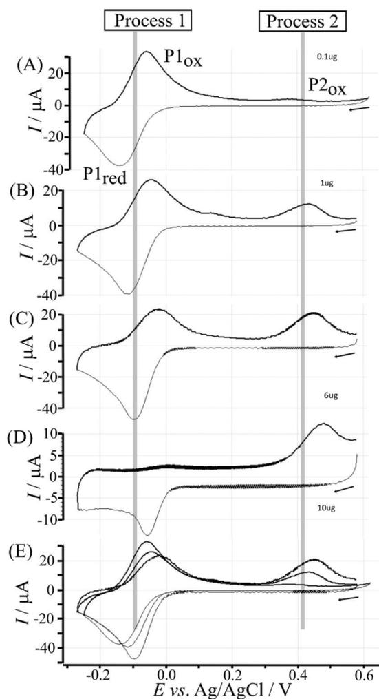
**Fig. 5** Cyclic voltammograms (scan rate  $100 \text{ mV s}^{-1}$ ) for T1-functionalised electrode with poly-NHG introduced onto the surface and immersed in phosphate buffer (0.1 M, pH 7) for (A) 0.1, (B) 1.0, (C) 6.0, and (D) 10  $\mu\text{g}$  T1. (E) Overlay of data from A to C.
