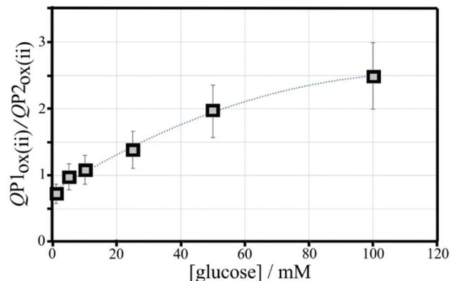
Fig. 10 Plot of the ratio of charges  $QP1_{ox}(ii)/QP2_{ox}(ii)$  versus glucose concentration for cyclic voltammetry experiments (scan rate  $50$  mV s $^{-1}$ ; poly-NHG from  $0.05$  mM solution;  $6$   $\mu$ g T1) in  $0.1$  M phosphate buffer pH 7. Polynomial line:  $-0.0001x^2 + 0.03x + 0.7649$ ; errors estimated  $\pm 20\%$ .
