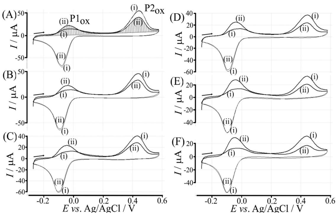
Fig. 9 Cyclic voltammograms (scan rate  $50$  mV s $^{-1}$ ; in  $0.1$  M phosphate buffer pH 7) for a  $6$   $\mu$ g T1-functionalised electrode with poly-(NHG) introduced onto the surface and immersed in (A)  $1$  mM, (B)  $5$  mM, (C)  $10$  mM, (D)  $25$  mM, (E)  $50$  mM, and (F)  $100$  mM glucose.
