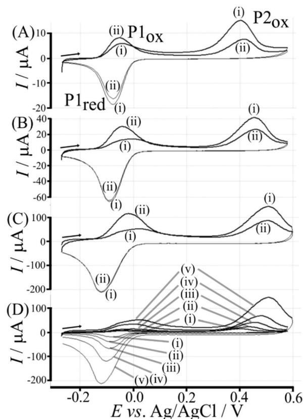
**Fig. 8** Cyclic voltammograms (scan rate (A) 10, (B) 50, (C) 200  $\text{mV s}^{-1}$ ; (D) overlay for (i) 10, (ii) 25, (iii) 50, (iv) 100, and (v) 200  $\text{mV s}^{-1}$ ) for a 6  $\mu\text{g}$  T1-functionalised electrode with poly-(NHG) introduced onto the surface and immersed in phosphate buffer (0.1 M, pH 7) with 50 mM glucose.
