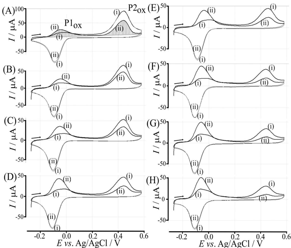
Fig. 11 Cyclic voltammograms (scan rate  $50 \text{ mV s}^{-1}$ ; in 0.1 M phosphate buffer pH 7) for a  $6 \mu\text{g}$  T1-functionalised electrode with poly-(NHG) introduced onto the surface and immersed in (A) 0.01 mM, (B) 0.1 mM, (C) 1 mM, (D) 5 mM, (E) 10 mM, (F) 25 mM, (G) 50 mM, and (H) 100 mM fructose.
