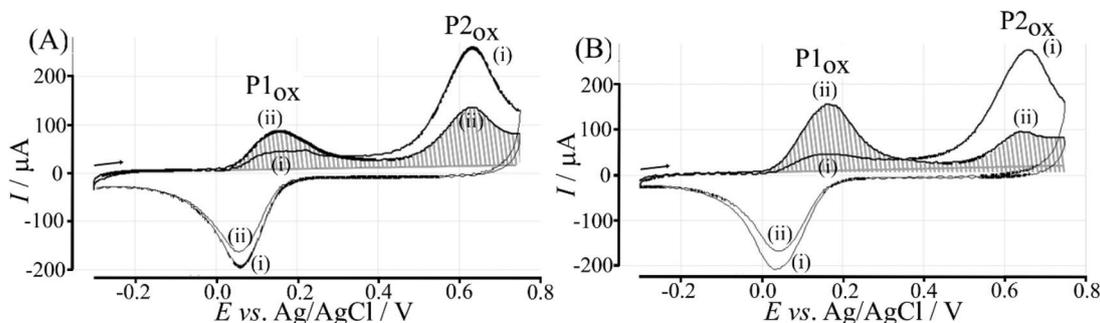
**Fig. 13** Cyclic voltammograms (scan rate  $100 mV s^{-1}$ ) for a T1 – functionalised graphene foam electrode with poly-NHG (0.1 mM) introduced onto the surface and immersed in human serum (4.9 mM glucose present in serum) spiked with (A) glucose to give a total concentration of 44.9 mM and (B) fructose to give a total concentration of 44.9 mM.
