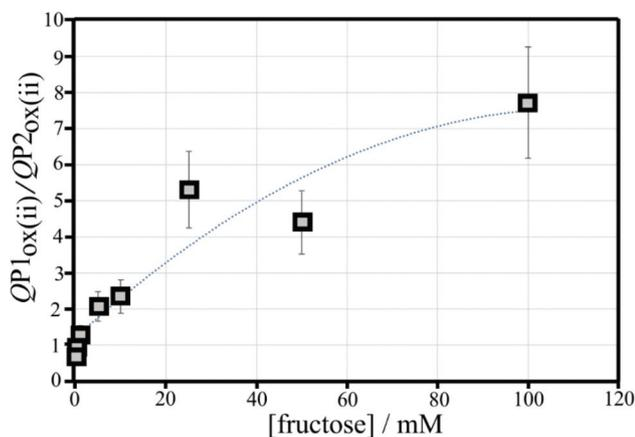
**Fig. 12** Plot of the ratio of charges  $QP1_{ox(ii)}/QP2_{ox(ii)}$  versus fructose concentration for cyclic voltammetry experiments (scan rate  $50 mV s^{-1}$ ; poly-NHG from 0.05 mM solution;  $6 \mu g T1$ ) in 0.1 M phosphate buffer pH 7. Polynomial line:  $-0.0005x^2 + 0.1142x + 1.21$ ; errors estimated  $\pm 20\%$ .
