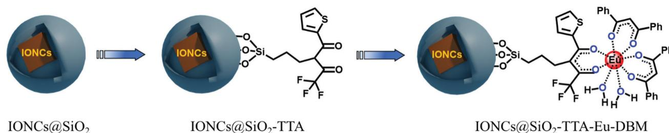
**Scheme 1** Illustration of each step of the functionalization of the IONCs@SiO<sub>2</sub> nanomaterial.
