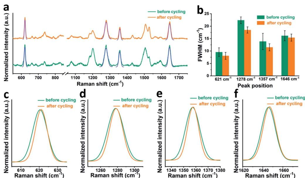
Fig. 3 (a) *Ex situ* SERS of RhB on a gold working electrode. (b) Comparison of the FWHM of Raman bands of RhB before and after cycling. Finally, we show in detail the following RhB Raman peaks with or without cycling: (c) 621 cm<sup>-1</sup>, (d) 1278 cm<sup>-1</sup>, (e) 1357 cm<sup>-1</sup> and (f) 1646 cm<sup>-1</sup>.
