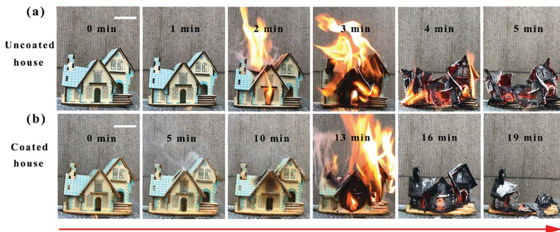
Fig. 4 Application of the biogel coating on wooden house models. Wooden house models without (a) and with (b) the biogel coating during combustion. Scale bar, 5 cm.
