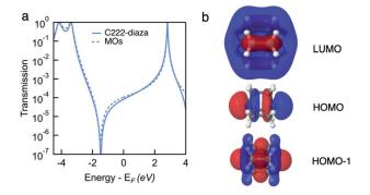
Fig. 4 (a) Transmission functions of C222-diaza, calculated as T(E) = $|t_{LUMO} + t_{HOMO} + t_{HOMO-1}|^2$  (dashed line) overlaid with Landauer transmission in the wide-band limit (solid). (b) MOs of C222-diaza calculated using DFT with B3LYP functional. White, black and blue atoms represent H, C and N, respectively.
