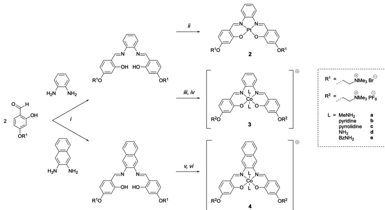
**Scheme 1** Synthesis routes to complexes **2**, **3a–3e** and **4a–4e**. [i] EtOH, reflux, 5 h,  $N_2$ ; [ii]  $K_2PtCl_4$ , DMSO, 65 °C, 18 h,  $N_2$ ; [iii]  $Co(OAc)_2 \cdot 4H_2O$ , MeOH, r.t., 1 h,  $N_2$ ; [iv] 10 eq. axial ligand L, aq. sat.  $NH_4PF_6$ , MeOH, r.t., 3 h, air; [v]  $Co(OAc)_2 \cdot 4H_2O$ , MeOH, r.t., 1 min, air; [vi] 10 eq. axial ligand L, aq. sat.  $NH_4PF_6$ , MeOH, r.t., 5 h, air.
