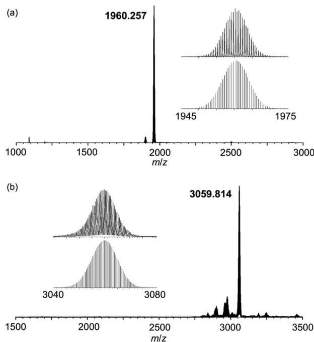
Fig. 3 Positive-ion ESI-mass spectra of (a) **I** and (b) **II** in acetonitrile. Insets: (a) spectrum in the range of  $m/z$  1945–1975, and simulated patterns for  $[\text{TPP}_6\text{HPMo}_9\text{O}_{37}\text{Mn}_4(\text{OAc})_3]^{2+}$  ( $m/z$ : 1960.262); (b) spectrum in the range of  $m/z$  3040–3080 and simulated patterns for  $[\text{TPP}_8\{\text{Mn}(\text{acac})_2\text{Mn}_4(\text{PMo}_9\text{O}_{34})_2\}]^{2+}$  ( $m/z$ : 3059.837).
