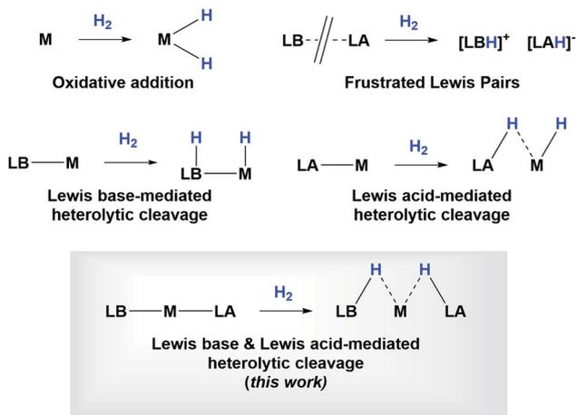
Fig. 8 Different types of H<sub>2</sub> activation.
