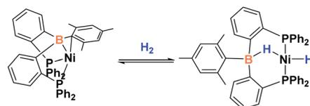
Scheme 1 Activation of H<sub>2</sub> by a nickel–borane complex.
