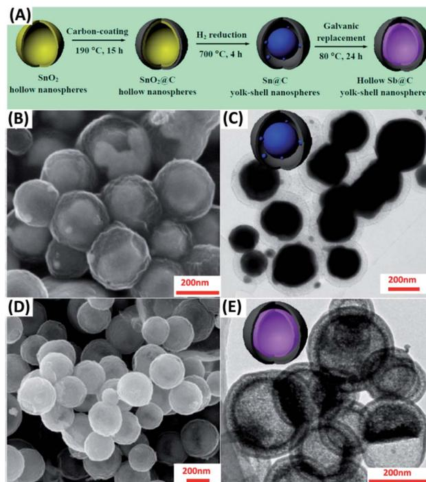
Fig. 2 (A) Synthetic approach to Sb–C yolk–shell nanostructures by galvanic replacement. (B and C) SEM and TEM images for Sn–C. (D and E) SEM and TEM images for Sb–C. Reproduced with permission from ref. 67. Copyright 2017, American Chemical Society.
