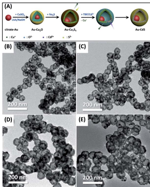
Fig. 1 (A) Synthetic approach to Au–CdS yolk–shell nanostructures by Kirkendall effect. (B–E) TEM images of Au–CdS with increasing void sizes. Reproduced with permission from ref. 63. Copyright 2019, Elsevier.
