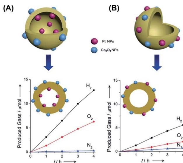
Fig. 15 Comparative results of photocatalytic water splitting under UV illumination on C<sub>3</sub>N<sub>4</sub> hollow structures with (A) spatially separate co-catalysts and (B) randomly distributed co-catalysts. Reproduced with permission from ref. 138. Copyright 2016, Wiley.
