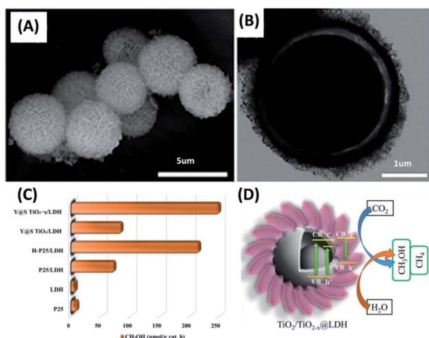
Fig. 8 (A and B) SEM and TEM images of Y@S-TiO<sub>2-x</sub>/LDH. (C) Comparative results of CO<sub>2</sub> reduction in terms of CH<sub>3</sub>OH production under visible light illumination. (D) Plausible charge transfer mechanism for superior photocatalytic efficiency of Y@S-TiO<sub>2-x</sub>/LDH toward CO<sub>2</sub> reduction. Reproduced with permission from ref. 98. Copyright 2019, American Chemical Society.
