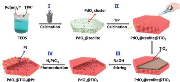
Fig. 16 Schematic illustration of using zeolites as structurally confined template to achieve spatial separation of dual co-catalysts on  $\text{TiO}_2$ . Reproduced with permission from ref. 137. Copyright 2020, American Chemical Society.
