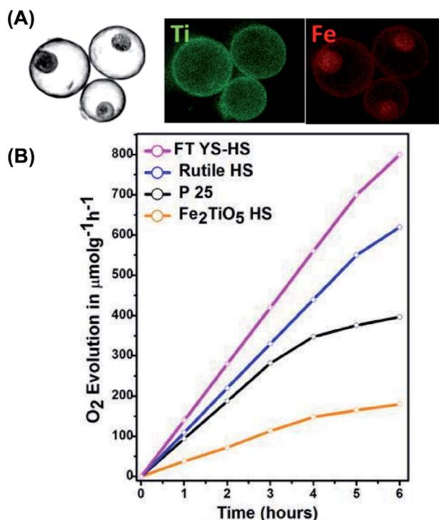
Fig. 10 (A) HAADF scanning TEM image and the corresponding EDS data of FTYS-HS, (B) comparative results of O<sub>2</sub> production under white light illumination. Reproduced with permission from ref. 104. Copyright 2017, Elsevier.
