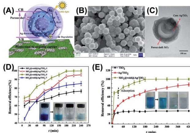
Fig. 6 (A) Plausible charge transfer mechanism for superior photocatalytic efficiency of  $\text{Ag}/\text{TiO}_2\text{-SiO}_2$  toward MB degradation, (B and C) SEM and TEM images of  $\text{Ag}/\text{TiO}_2\text{-SiO}_2$ , (D) photocatalytic performance of  $\text{Ag}/\text{TiO}_2\text{-SiO}_2$  prepared with the removal of different Ppy layers, (E) comparative results of MB degradation under visible light illumination. Reproduced with permission from ref. 83. Copyright 2019, Elsevier.
