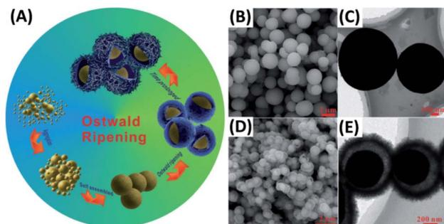
Fig. 3 (A) Synthetic approach to N-doped TiO<sub>2</sub>-C yolk-shell spheres by Ostwald ripening. (B and C) SEM and TEM images for solid TiO<sub>2</sub>. (D and E) SEM and TEM images for N-doped TiO<sub>2</sub>-C. Reproduced with permission from ref. 72. Copyright 2016, Wiley.
