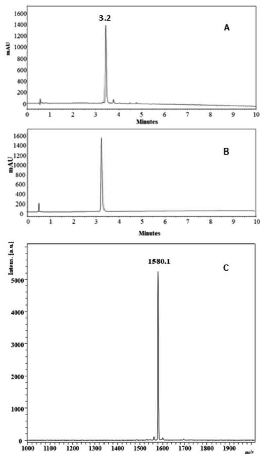
Fig. 1 Analytical characterization of peptide 2: C-Ahx-SPINNTK-PHEAR. Chromatographic profile of the crude (A) and pure product (B). MALDI-TOF MS spectrum of pure peptide (C), signal at  $m/z$  1580.1 corresponds to the  $[M + H]^+$  species.
