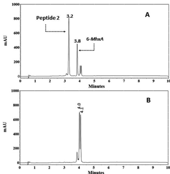
Fig. 6 Monitoring via RP-HPLC of the reaction in solution between peptide 2 (C-Ahx-SPINNTKPHEAR) and the 6-maleimidoheptanoic acid (6-MhxA). Reaction time: 1 min (A) and 24 hours (B).
