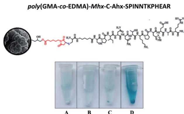
Fig. 8 Antigen-antibody interaction assays of functionalized monolithic material. (A) Post-IV serum incubated in the absence of a monolith; (B) post-IV serum incubated with poly(GMA-co-EDMA); poly(GMA-co-EDMA)-Mhx-C-Ahx-SPINNTKPHEAR incubated with preimmune serum, PI (C) or post-IV serum (D).
