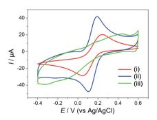
Fig. 2 CVs obtained from different modified electrodes in 5 mM  $[Fe(CN)_6]^{3-/4-}$  solution containing 0.1 M KCl and 0.1 M PBS at a scan rate of 100 mV s<sup>-1</sup>. (i) GCE, (ii) rGO/GCE, (iii) Hemin-doped-HKUST-1/rGO/GCE.
