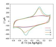
Fig. 3 CVs obtained at different modified electrodes in 0.10 M PBS at a scan rate of 100 mV s<sup>-1</sup>. (i) rGO/GCE, (ii) Hemin/rGO/GCE, (iii) HKUST-1/rGO/GCE and (iv) Hemin-doped-HKUST-1/rGO/GCE.
