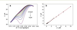
Fig. 6 (a) DPV of the Hemin-doped-HKUST-1/rGO/GCE in 0.1 M PBS with different concentrations of DA (0.03–10  $\mu$ M). (b) Calibration plots of the redox peak currents against different concentrations of DA.
