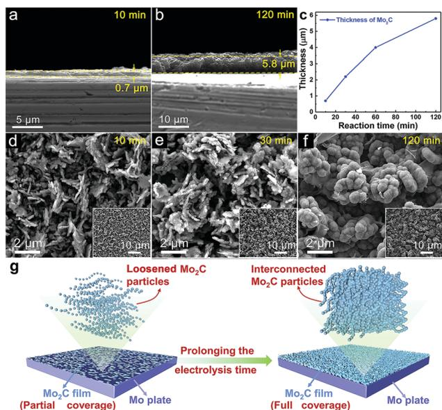
Fig. 4 Cross-sectional SEM images of  $\text{Mo}_2\text{C}/\text{Mo}$ -10 (a) and  $\text{Mo}_2\text{C}/\text{Mo}$ -120 (b). (c) Thickness change of the  $\text{Mo}_2\text{C}$  layer vs. electrolysis time. SEM images of  $\text{Mo}_2\text{C}/\text{Mo}$ -10 (d),  $\text{Mo}_2\text{C}/\text{Mo}$ -30 (e) and  $\text{Mo}_2\text{C}/\text{Mo}$ -120 (f). (g) Illustration of the changes of thickness and morphology of the  $\text{Mo}_2\text{C}$  film by prolonging the electrolysis time.
