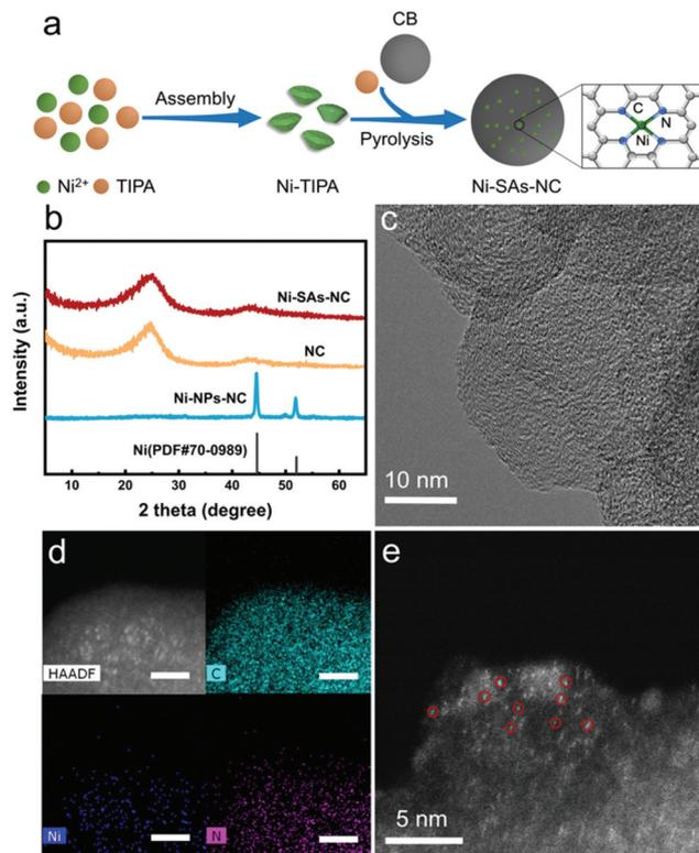
**Fig. 1** (a) The schematic illustration of the preparation of Ni-SAs-NC. (b) PXRD patterns of Ni-SAs-NC, Ni-NPs-NC and NC. (c) TEM and (d) EDX elemental mapping images of Ni, C and N elements of Ni-SAs-NC (scale bar = 5 nm). (e) HAADF-STEM image of Ni-SAs-NC.
