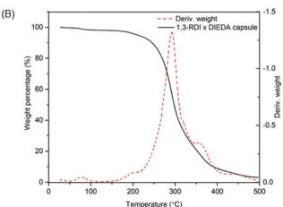
Fig. 5 TGA weight loss profiles and their first derivatives of (A) 1,3-ArDI-DIEDA capsules and (B)1,3-RDI-DIEDA capsules.
