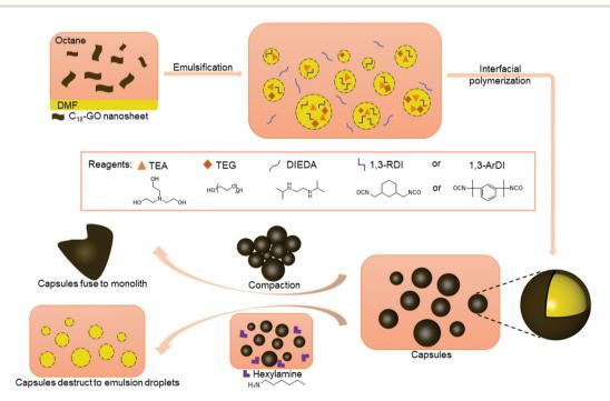
Scheme 1 Overview of the work reported here: formation of capsules with shells containing hindered urea bonds (HUBs) and the fusion or destruction of the capsule shells. Capsules were prepared by interfacial polymerization in oil-in-oil Pickering emulsions stabilized by functionalized graphene oxide nanosheets.
