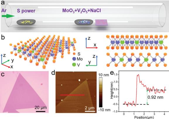
Fig. 1 (a) Schematic of synthesis of V-doped  $MoS_2$  by CVD. (b) Atom structure and side view of V-doped  $MoS_2$ . (c) Optical image of a V-doped  $MoS_2$  single crystal. (d and e) AFM topography and thickness measurement of V-doped  $MoS_2$ .
