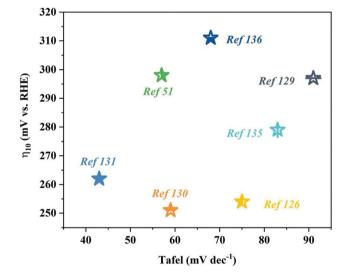
Fig. 15 OER activity comparison graph showing the Tafel slope versus overpotential at a current density of 10 mA  $\rm cm^{-2}$  for different catalysts.
