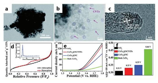
Fig. 21 (a and b) TEM images of CoTe<sub>2</sub>@NCNTFs. (c) HRTEM image of CoTe<sub>2</sub>@NCNTFs. (d)  $N_2$  adsorption—desorption isotherms and the corresponding pore size distribution (inset) of CoTe<sub>2</sub>@NCNTFs. (e) CoTe<sub>2</sub> polarization curves of different catalysts. (f) Histogram of the overpotential of different catalysts at 10 mA cm<sup>-2</sup>. <sup>165</sup> Copyright © 2018, Royal Society of Chemistry.
