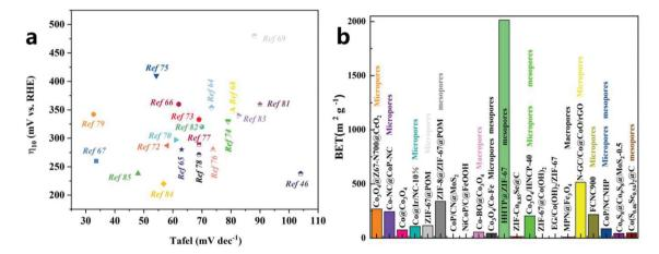
Fig. 6 (a) OER activity comparison graph showing the Tafel slope at an overpotential of 10 mA cm<sup>-2</sup> for different catalysts. (b) Comparison of BET/ BJH results for different catalysts.
