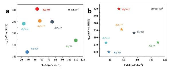
Fig. 11 OER activity comparison graph showing the Tafel slopes versus overpotential at current densities of 10 mA cm<sup>-2</sup> (a) and 100 mA cm<sup>-2</sup> (b) for different catalysts.
