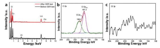
Fig. 12 (a) EDS analysis of Cl-doped  $\alpha$ -Co(OH)<sub>2</sub> catalyst in 1 M KOH solution. Cl 2p XPS spectra of the catalyst before OER test (b) and after the OER test (c).51 Copyright © 2019, Royal Society of Chemistry.
