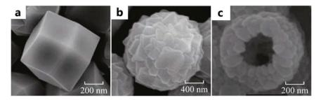
Fig. 1 SEM images of (a) T-ZIF-67, (b) M-ZIF-67, and (c) H-ZIF-67. Copyright @2017, The Author(s).
