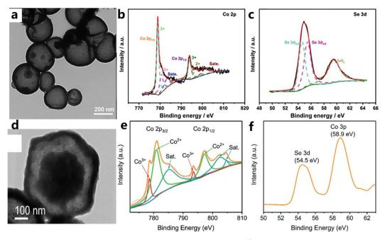
Fig. 20 (a) TEM image of CoSe<sub>2</sub>-30. (b) Co 2p and (c) Se 3d XPS spectra of CoSe<sub>2</sub>-30.<sup>49</sup> Copyright © 2019 Elsevier B.V. All rights reserved. (d) HR-TEM image of Y-S Ni-Co-Se. XPS spectra of the (e) Co 2p and (f) Se 3d regions.<sup>164</sup> Copyright @ 2018, American Chemical Society.
