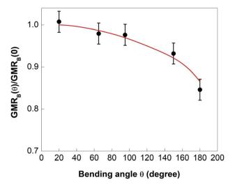
Fig. 7 Experimental  $\mathsf{GMR_B}(\theta)$  ratio (dots) normalized to the value measured on the flat sample ( $\theta=0^\circ$ ). Calculated values using eqn (1) are marked by a red line.
