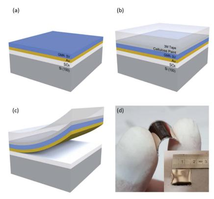
Fig. 2 (a–c) Sketch of the Au-mediated transfer-and-bonding approach: (a) perpendicular GMR-SVs are DC sputtered on a  $SiO_x/Si(100)$  substrate covered with a weakly adhering Au underlayer; (b) a cellulose paint is spread over the film surface to improve the adhesion between the sample and the adhesive tape on which the stack is transferred by a mechanical peel-off step (c). (d) Optical photograph of a flexible perpendicular GMR-SV ( $t_{Cu} = 3$  nm).
