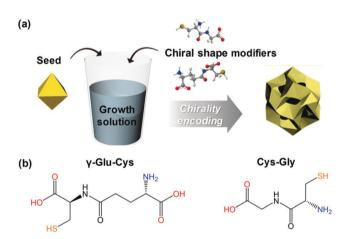
Fig. 6 (a) A schematic diagram indicating the preparation of chiral shape modifier-induced Au nanoparticles formation. (b) Chemical structures of the dipeptides are used as chirality inducers. Reprinted with permission.<sup>87</sup> Copyright 2020, Wiley-VCH.
