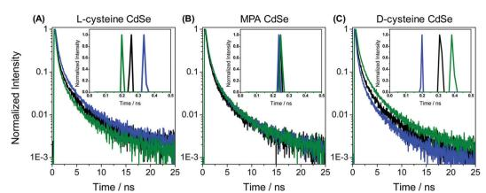
Fig. 16 (A-C) Lifetime decay profiles for acceptor CdSe QD functionalized with chiral L-cysteine, achiral mercaptopropionic acid, and chiral D-cysteine, respectively. Data represented in black, blue, and green correspond to the linear, clockwise, and counter-clockwise circularly polarized excitation light, respectively. Insets show the short parts of the lifetime distributions. Reprinted with permission. 108 Copyright 2017, American Chemical Society.
