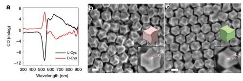
Fig. 5 (a) Visible-region CD spectra recorded on the L/D-cysteine-induced chiral metallic Au NPs. (b) SEM images of L-cysteine, and (c) D-cysteine induced chiral Au NPs. Reprinted with permission.<sup>88</sup> Copyright 2020, Springer Nature.
