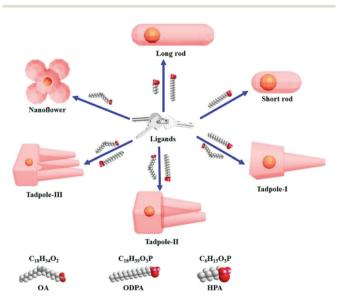
**Fig. 8** A schematic diagram showing that chiral ligand-induced shape variations resulting in various anisotropic shapes can be achieved. Chemical structures of the chiral ligands are shown. Reprinted with permission. <sup>91</sup> Copyright 2020, American Chemical Society.
