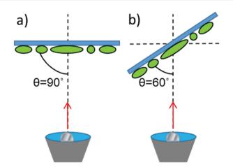
Fig. 2 Schematic for metal evaporation (a) Normal evaporation (b) Glancing angle evaporation. Note that the ellipsoids major axis alignment on the substrate is uncontrolled (see Fig. 3).
