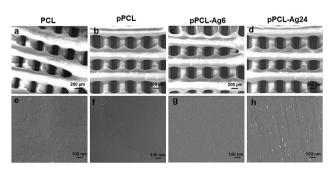
Fig. 2 SEM images of PCL, pPCL-Ag6, and pPCL-Ag24 at (a-d) lower and (e-h) higher magnifications.
