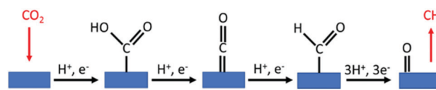
Fig. 27 A postulated mechanism of methane formation from the electrochemical reduction of CO 2 . Adapted with permission from ref. 199. Copyright (2015) American Chemical Society.
