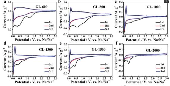
Fig. 26 CVs of HC samples pyrolysed at (a) 600, (b) 800, (c) 1000, (d) 1300, (e) 1500 and (f) 2000 °C. 107 Copyright 2019, Wiley.
