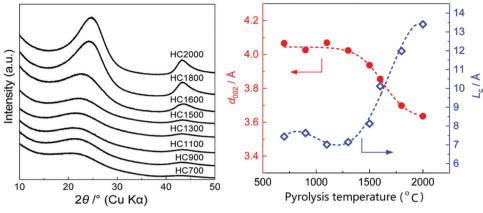
Fig. 18 (a) XRD patterns of sucrose-derived HC samples pyrolysed at temperatures between 700 and 2000 °C, and (b) relationship between d-spacing and graphitic crystallite length along the c-axis as a function of pyrolysis temperature.<sup>84</sup> Copyright 2020, American Chemical Society.
