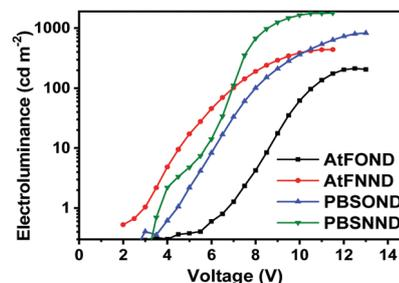
Fig. 9 Voltage dependency of electroluminescence (cd m<sup>-2</sup>) of NIR OLEDs.
