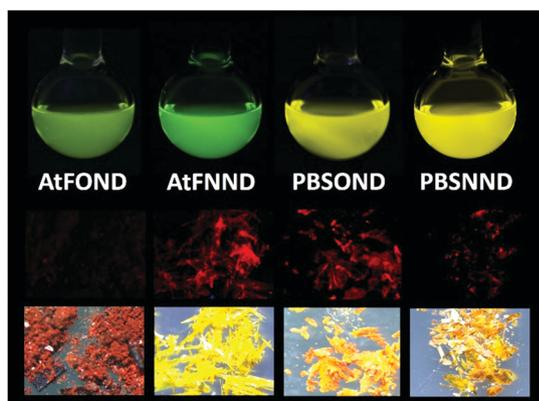
Fig. 2 Solution and solid images of **AtFOND**, **AtFNND**, **PBSOND**, and **PBSNND** (from the left to right). Top row: in a degassed dilute dichloromethane solution of  $1 \times 10^{-5}$  M. Crystals or non-crystalline powders obtained from a solution process of a single crystal grown under 365 nm UV (centre row) and under ambient conditions (bottom row).
