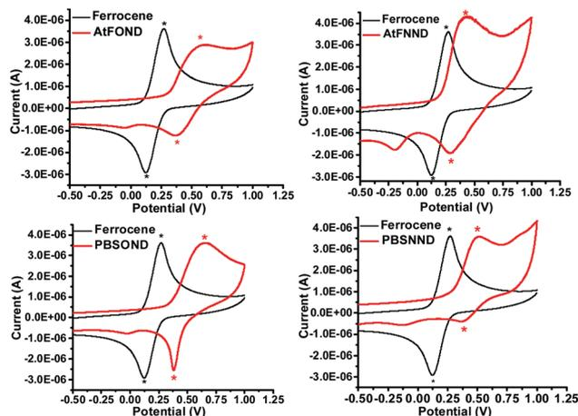
Fig. 6 Cyclic voltammograms of AtFOND, AtFNND, PBSOND, BSND, and ferrocene (reference) in  $\text{CH}_2\text{Cl}_2$  (1 mM) in the presence of 0.1 M TBAPF<sub>6</sub> at 295 K.
