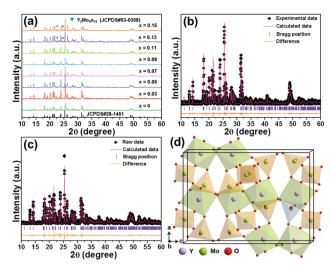
Fig. 1 (a) XRD patterns of the  $Y_2Mo_3O_{12}$ : $Er^{3+}/2xYb^{3+}$  microparticles. Rietveld XRD refinement patterns of the (b)  $Y_2Mo_3O_{12}$ : $Er^{3+}$  and (c)  $Y_2Mo_3O_{12}$ : $Er^{3+}/0.22Yb^{3+}$  microparticles. (d) Crystal structure of the  $Y_2Mo_3O_{12}$  unit cell.
