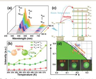
Fig. 3 (a) Temperature-dependent UC emission spectra and (b) emission intensities of the  $Y_2Mo_3O_{12}$ : $Er^{3+}/0.22Yb^{3+}$  microparticles. (c) Energy level diagram illustrating thermally promoted ET from Yb3+ to Er3+ ions. (d) CIE coordinate diagram of the  $Y_2Mo_3O_{12}$ : $Er^{3+}/0.22Yb^{3+}$  microparticles as a function of temperature. The inset shows the optical images of the resultant samples at different temperatures excited at 980 nm.
