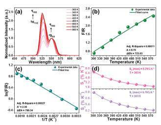
Fig. 4 (a) Normalized green UC emission spectra of the  $Y_2Mo_3O_{12}$ :Er<sup>3+</sup>/ 0.22Yb<sup>3+</sup> microparticles in the temperature range of 303–583 K. (b) Temperature-dependent FIR value. (c) Plot of In(FIR) *versus* 1/T of the  $Y_2Mo_3O_{12}$ :Er<sup>3+</sup>/0.22Yb<sup>3+</sup> microparticles. (d) Dependence of the  $S_a$  and  $S_r$  values on the temperature.
