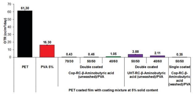
Fig. 3 OTR values of PET, PVA, Cop-RC-β aminobutyric acid/PVA/PET film (green) and UHT-RC-β-aminobutyric acid/PVA/PET (purple) film with a coating mixture at 5 wt% solid content. Double layer coated film with a coating mixture containing unwashed LDHs/PVA at various ratios. Single layer coated film with a coating mixture containing washed Cop-RC-\u00b3-aminobutyric acid/PVA at the ratio of 50/50 (blue).
