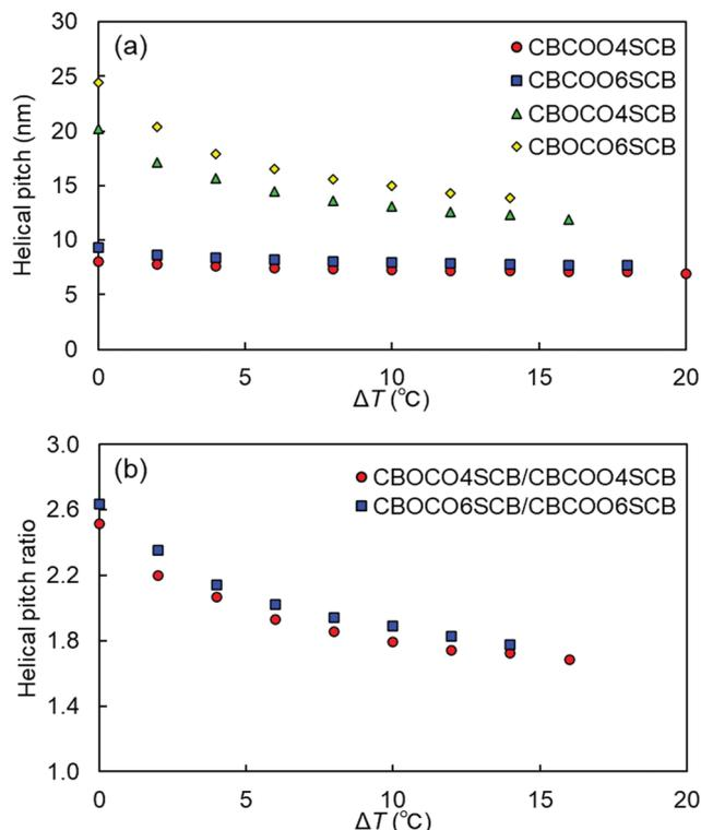
Fig. 6 (a) Helical pitches of CBCOO4SCB, CBCOO6SCB, CBOCO4SCB, and CBOCO6SCB, and (b) helical pitch ratios of CBOCO4SCB/CBCOO4SCB and CBOCO6SCB/CBCOO6SCB as a function of the shifted temperature ( $\Delta T = T_{\text{NNTB}} - T$ ).
