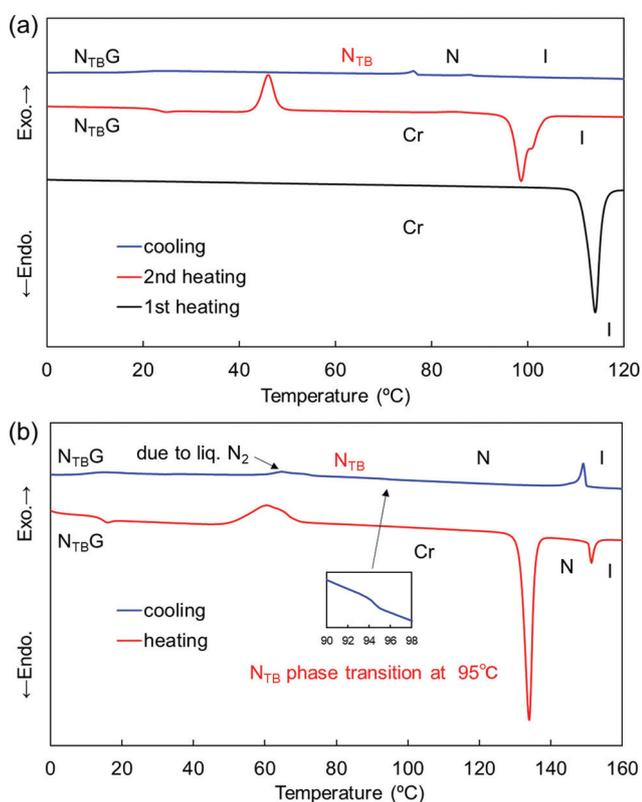
**Fig. 2** DSC curves of (a) CBCOO6SCB and (b) CBOCO6SCB recorded at a rate of 10 °C min<sup>-1</sup>.
