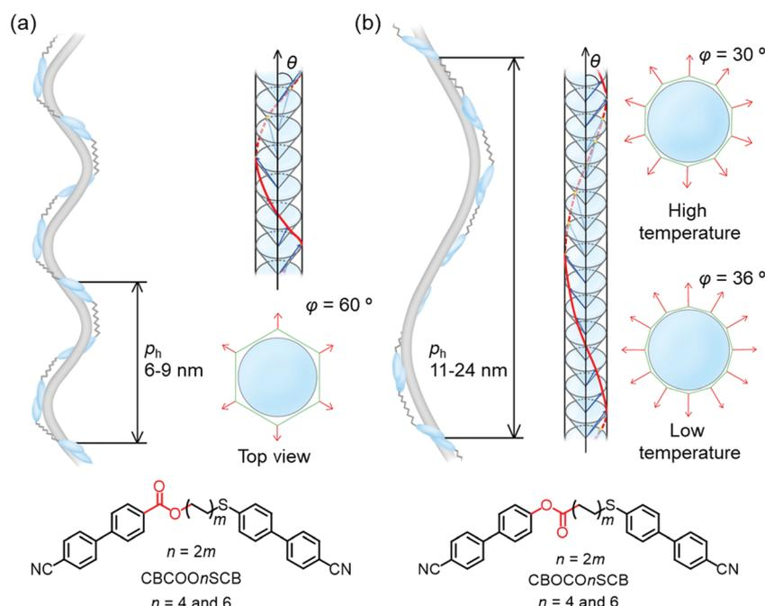
Fig. 7 Plausible helical helix models in the  $N_{\text{TB}}$  phases of (a) CBCOO4SCB and CBCOO6SCB, and of (b) CBOCO4SCB and CBOCO6SCB.
