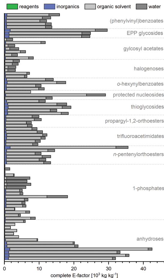
Fig. 4 Complete E-factors of nearly all routes are mainly composed of solvent contributions. All contributions are also given in the ESI† with reference to the procedure and details for calculation.
